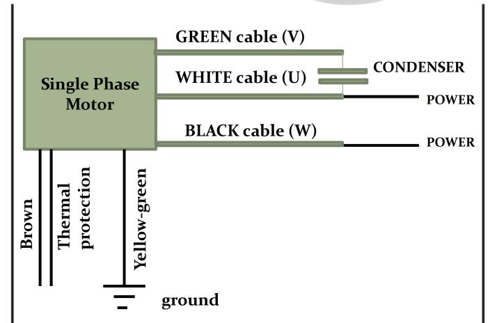
Thermistor brown wires to be connected to the amplifier operating voltage = 2.5V
